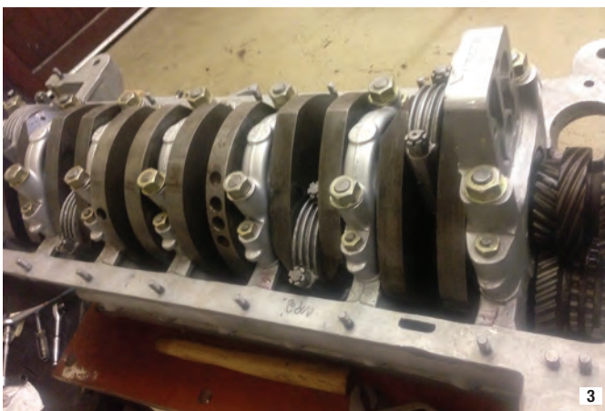
1, Assembling the parts to build the 3.5 litre straight six engine. The crankshafts were machined from a solid billet of steel and weighed around 50kgs, more than the aluminium engine block.
